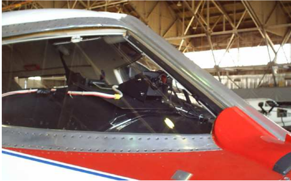
Figure 3.5: A Dalsa Pantera TF 1M60 monochrome digital camera provided by AFRL was mounted on the glare shield of the simulated receiver, a Calspan Learjet LJ-24.
