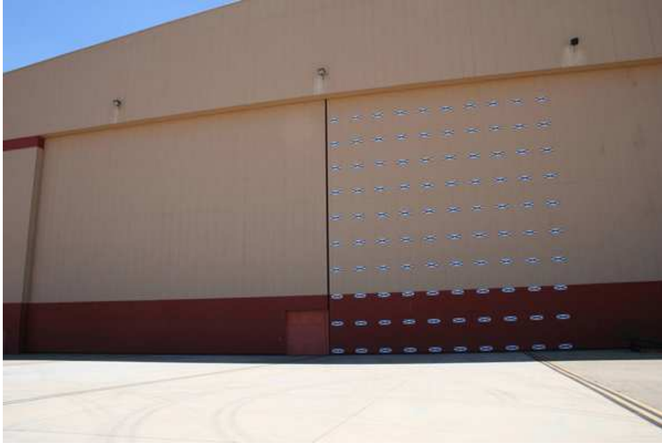
Figure 3.6: The setup of the camera calibration for the flight tests.
